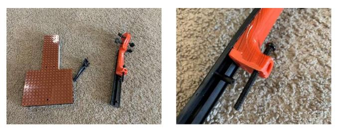
Step 2b Put the screw into the upper middle hole as marked.
